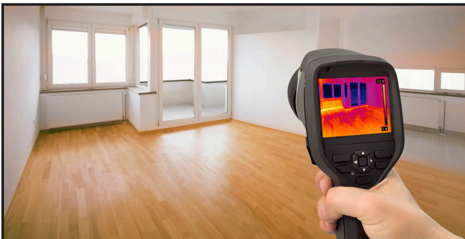
An infrared detector is taking an image of the heat loss in the room, which is indicated by the colour; red being hotter and blue cooler. The image clearly shows the heat loss through the windows and doors.
